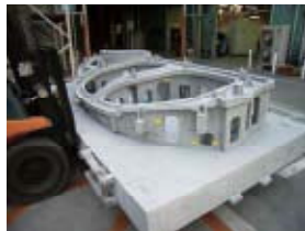
Jig for inspection of side-panel parts of automobile
