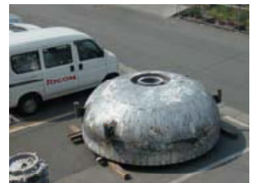
Example of ultra-large-scale casting (diameter exceeding 3m)
