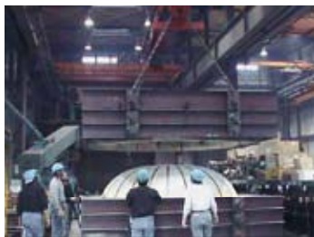
Casting of large-scale aluminum casting using large-scale mold rolover machine developed in-house.
